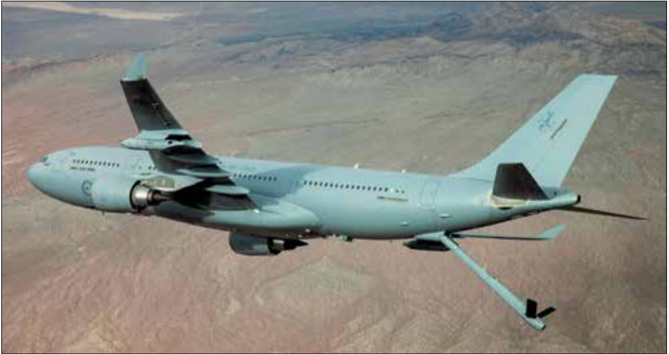
An Airbus KC-30A of No 33 Squadron during boom refuelling trials in the United States, October 2015. Source: Department of Defence
