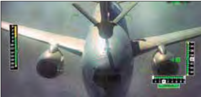
A Boeing E-7A Wedgetail of No 2 Squadron refuelling from the boom of an Airbus KC-30A of No 33 Squadron as seen through the KC-30A's Air Refuelling Operator's flight deck refuelling station screens in the skies over Iraq during Operation Okra . Source: Department of Defence
