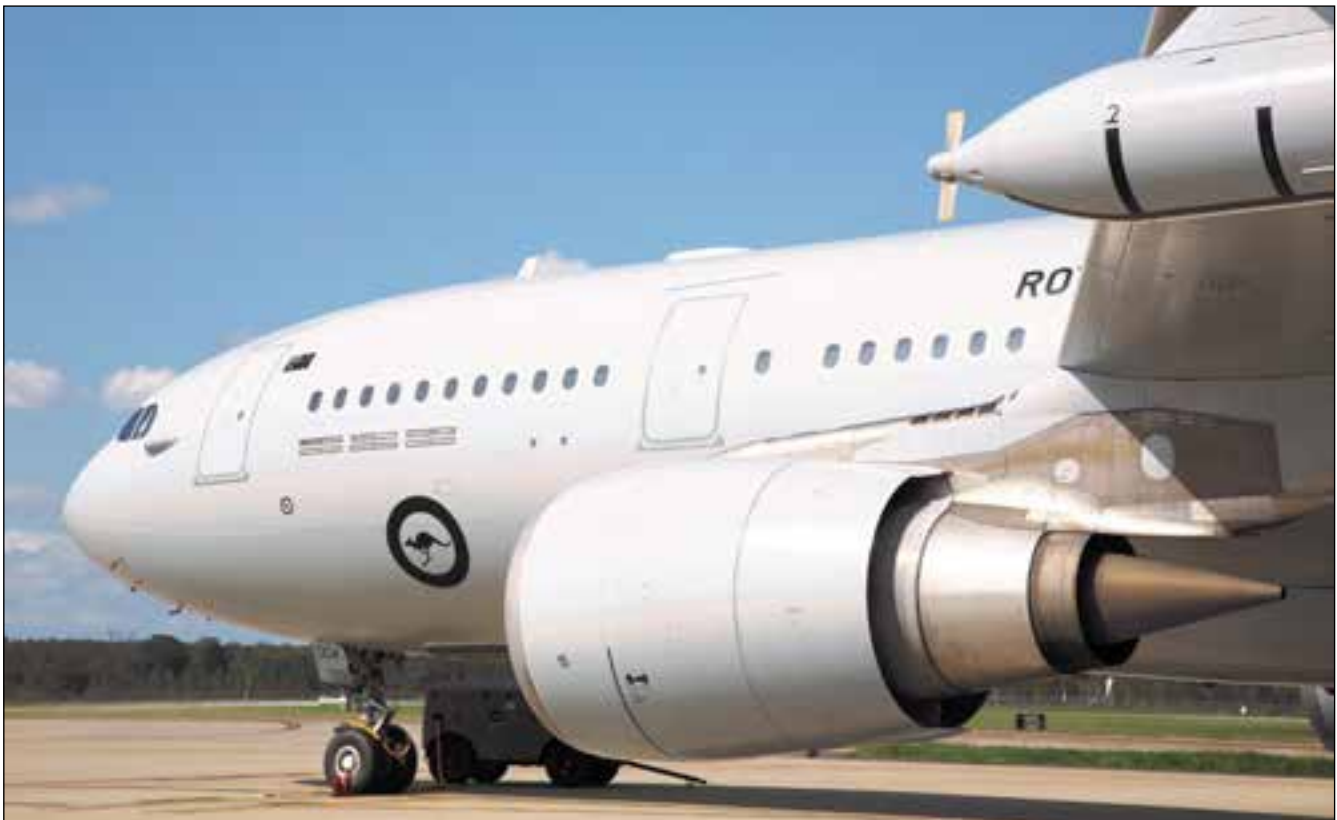
The nose and port engine of a No 33 Squadron Airbus KC-30A, with the front of the port drogue refuelling pod visible top right. Source: Department of Defence
